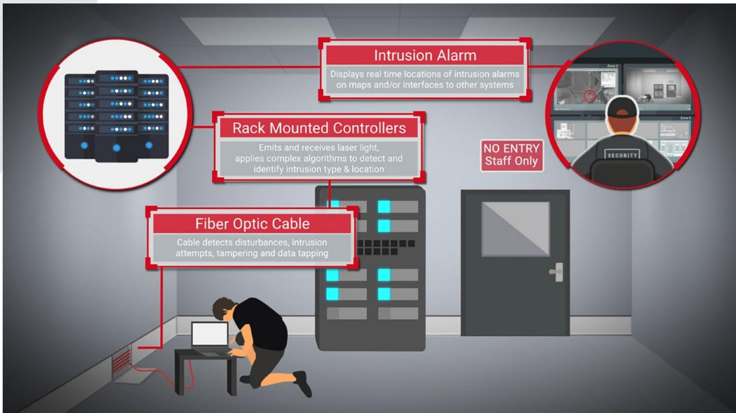
FFT's fibre optic technology is designed to detect and locate disturbances, intrusion attempts, tampering, and data tapping activities to within 5 metres along data networks. This can be applied anywhere from local data centre LANs to long distance WAN transport reaching thousands of kilometres in length.
